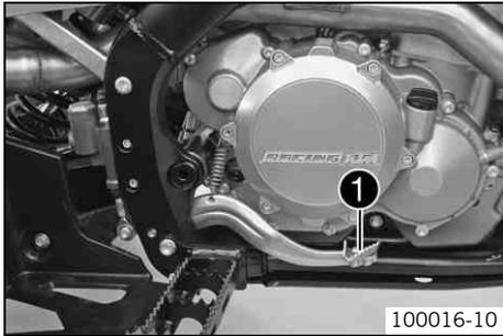
The foot brake lever ❶ is located in front of the right footrest.
