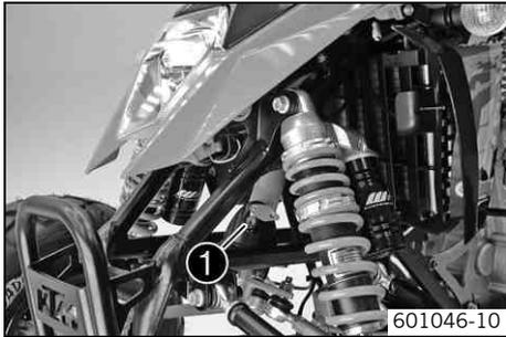
The steering lock ❶ is fitted on the steering column.
