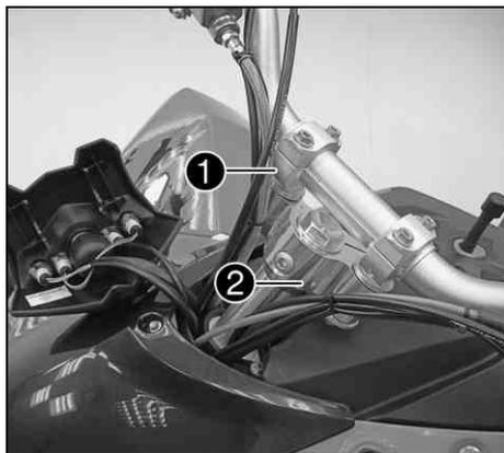
The handlebar position can be adjusted 4-fold by turning the handlebar support **1** and the handlebar support **2**.
