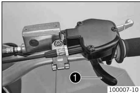
The throttle lever ❶ is fitted on the right side of the handlebar. The throttle lever is used to control the engine speed.
