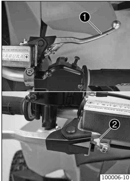
The hand brake lever ❶ is located on the right side of the handlebar and operates the front brakes.
