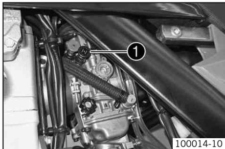
The choke ❶ is fitted on the left side of the carburetor. Activating the choke function frees an opening through which the engine can draw extra fuel. This gives a richer fuel-air mixture, which is needed for a cold start.
