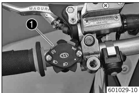
The kill switch ❶ is fitted on the left side of the handlebar.
