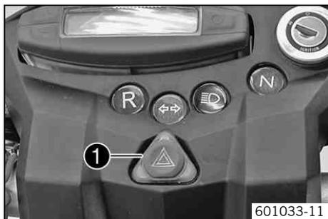
The hazard warning flasher switch ❶ is fitted centrally below the indicator lamps. The hazard warning flasher is used to indicate emergency situations.
