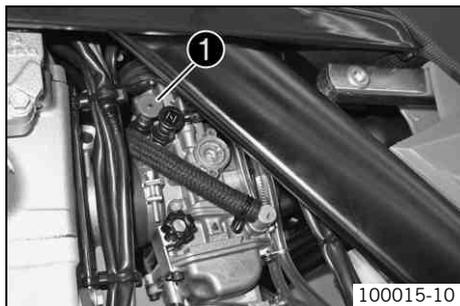
The hot start button (red) ❶ is fitted on the left side of the carburetor. Activating the hot start function frees an opening in the carburetor through which the engine can draw extra air. This gives a leaner fuel-air mixture, which is needed for a hot start.
