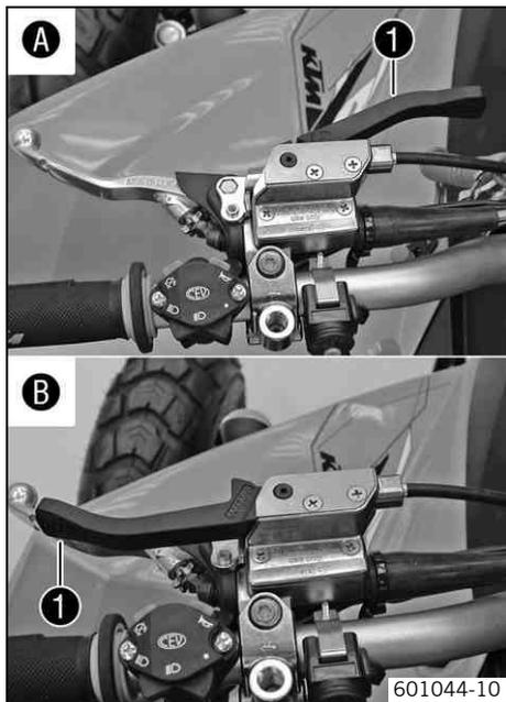
The parking brake lever ❶ is located on the left side of the handlebar and operates the rear brakes.
