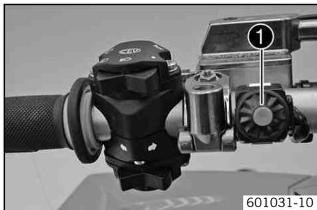
The electric starter button ❶ is fitted on the left side of the handlebar.
