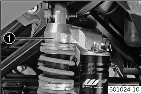
The shock absorber part number ❶ is stamped on the top part of the shock absorber.
