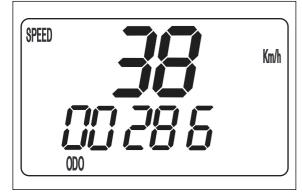
The ODO mode shows the speed and the total kilometers traveled. The information will disappear in the display when the front wheel stops turning for 1 minute.
