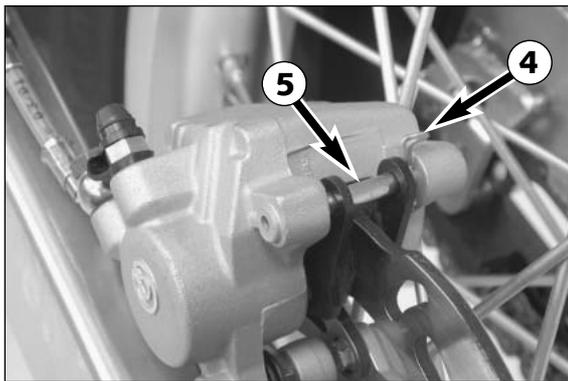
Slide left brake pad into the brake caliper and fix it with the pin. Slide in the right brake pad and knock the bolt in as far as it will go. Mount safety device ④.
