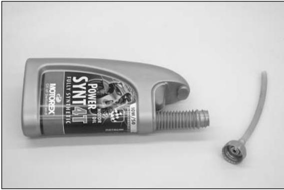
To facilitate bleeding of the oil system, we have added a hose connection piece and a plastic hose to the set of tools. Take an empty oil can (1 liter) and drill a 7 mm (0.28 in) -diameter hole into the lid. Screw the hose connection piece into the lid from the outside, and secure it from the inside with the M8 hexagon nut. Slip the plastic hose onto the hose connection piece, and you will have your filling tool.
