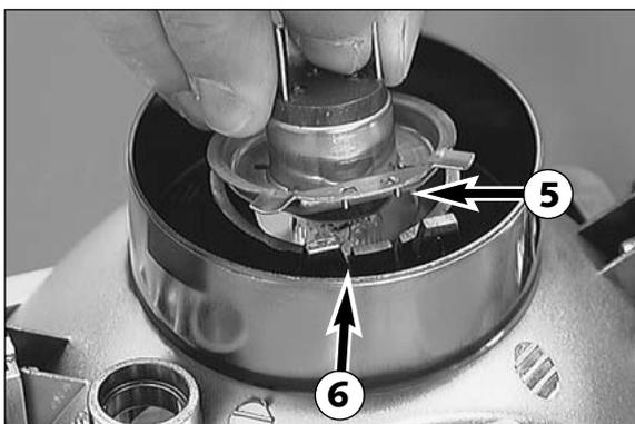
Insert the new lamp such that the noses **5** engage in the recesses **6**. When doing so, do not touch the glass body of the lamp so that it remains free from fat. Engage retaining clip, mount rubber cap and connector. If the parking-light lamp is to be replaced, simply insert it in the holder. Reinsert the parking-light lamp together with the holder.
