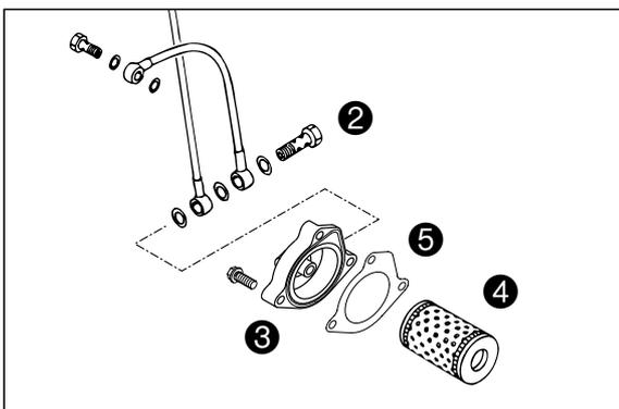
Place the new oil filter ④ on the connection in the oil filter cover and mount together with a new seal ⑤. Tighten the 3 screws in the filter cover to 5 Nm. Tighten the hollow screw with seals and tighten to 15 Nm. Finally, start the engine and check the oil system for leakage.
