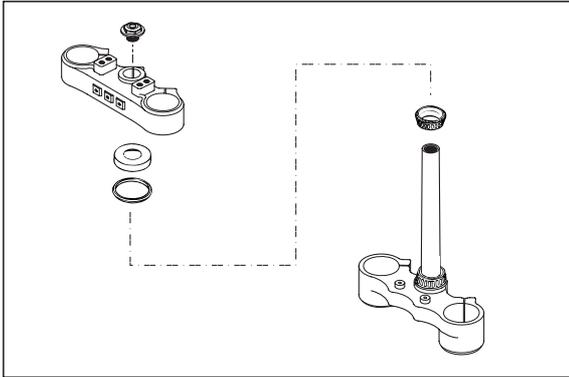
At least once a year, the steering head bearings should be smeared with waterproof grease (Motorex Long Therm 2000).
