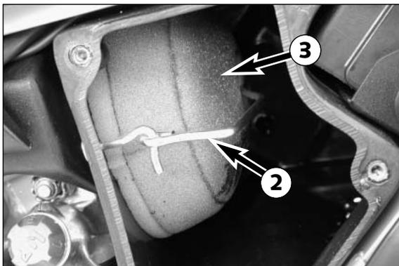
Remove the air filter from the filter holder and wash thoroughly in special cleaning fluid. Motorex offers environmentally-friendly products for professional oil filter maintenance (Motorex Bio Dirt Remover + Motorex Liquid Bio Power). Press out the water from the air filter but do not wring and allow the filter to dry. Lubricate the dry air filter thoroughly with highgrade filter oil, rubbing to coat the entire filter surface.
