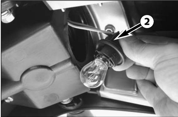
Turn the lamp socket ❷ approximately 30° counterclockwise and pull it out of the tail light housing.
