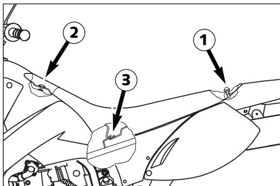
When installing the seat, be sure to insert the rear portion of the seat into the metal clasp ③.
