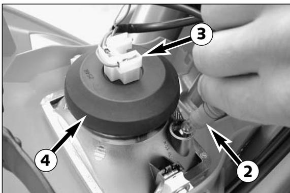
Pull the parking light lamp with holder **2** carefully out of the reflector. Pull connector **3** off the headlamp and remove rubber cap **4**. Disengage retaining clip and take bulb out of reflector. When changing the parking-light lamp, simply pull it out of the holder.
