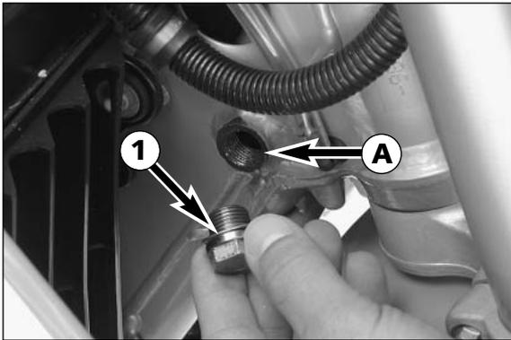
Fill 0.6 liters (0.16 US gallons) of engine oil into the can and remove the plug ① next to the steering head. Introduce the plastic hose into the vent hole ①, (see page 30) and fill 0.6 liters (0.16 US gallons) of engine oil into the frame's front tube. Remove plastic hose, start engine, and let it idle (approx. 20 seconds) until oil escapes at the hole ①. As soon as oil begins to leak out, switch off the engine, mount the plug and gasket and tighten to 25 Nm.
