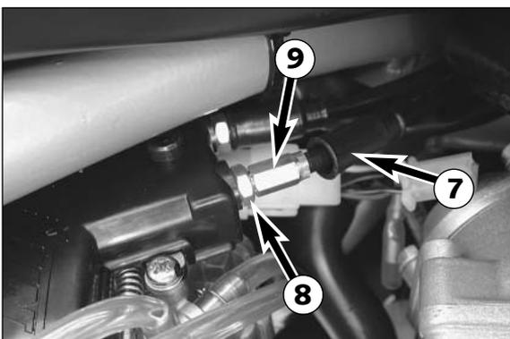
To adjust the throttle cable, push back the protection cover ⑦, loosen the counter nut ⑧ and turn the adjusting screw ⑨ as required. Turning the adjusting screw counterclockwise will reduce the backlash, turning the adjusting screw clockwise will increase the backlash.
