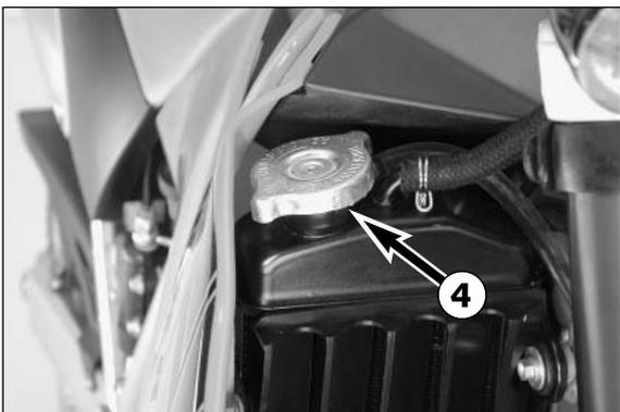
A mixture of 40% anti freeze liquid and 60% water is used as coolant. However, the anti-freeze protection must be at least -25° C (-13° F). This mixture offers anti-freeze protection but also good corrosion protection and should therefore not be replaced by pure water.
