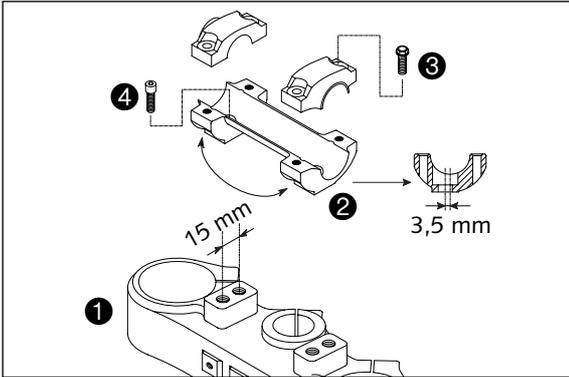
For this purpose, remove screws ❸ of the handlebar clamps and screws ❹ of the handlebar support. Position handlebar support, and tighten screws ❹ to 40 Nm (30 ft.lbs). Mount handlebar and handlebar clamps, and tighten screws ❸ to 20 Nm (15 ft.lbs). The gap between handlebar support and handlebar clamps is to be of equal size in the front and in the rear.
