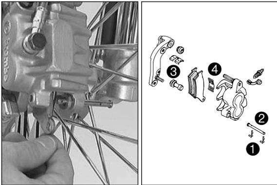
Mount the right brake pad and fix it with the bolt. Mount the left brake pad and insert the bolt until it stops. Mount the clips. When mounting the brake pads, be sure to check for correct fit of the sliding metal-sheet ③ in the caliper support and of the leaf spring ④.
