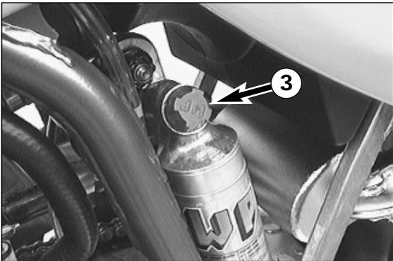
**Compression damping of shock absorber**
