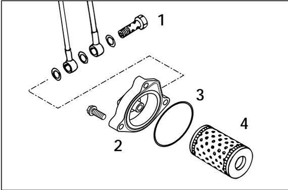
Check the O-ring ③ for damage. O-rings need not be replaced unless damaged. Press the O-ring into the groove of the filter cover. Fit new oil filter ④ with rubber gasket on the fitting in oil filter cover and mount cover with filter. Mount three screws and tighten with 5 Nm (4 ft.lb). Mount hollow screw with seal rings and tighten with 15 Nm (11 ft.lb). Start engine and check oil system for leakage.
