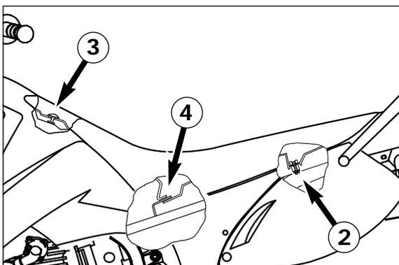
To mount the seat hook it into the oval head screw, lower the rear part of the seat and push the whole seat forwards. If necessary push the middle of the seat slightly down to let the retaining bracket ❹ engage with the seat. Finally fasten the seat with the corresponding screw.
