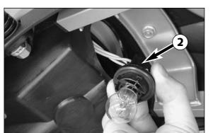
Turn the lamp socket 2 approximately 30° counterclockwise and pull it out of the tail light housing.
