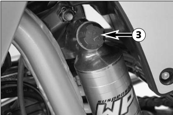
**Compression damping of shock absorber**
