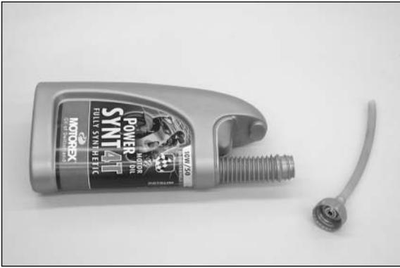
To facilitate bleeding of the oil system, we have added a hose connection piece and a plastic hose to the set of tools. Take an empty oil can (1 liter) and drill a 7 mm-diameter hole into the lid. Screw the hose connection piece into the lid from the outside, and secure it from the inside with the M8 hexagon nut. Slip the plastic hose onto the hose connection piece, and you will have your filling tool.
