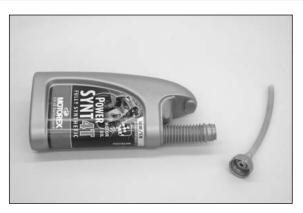
To facilitate bleeding of the oil system, we have added a hose connection piece and a plastic hose to the set of tools. Take an empty oil can (1 liter) and drill a 7 mm (0.28 in) -diameter hole into the lid. Screw the hose connection piece into the lid from the outside, and secure it from the inside with the M8 hexagon nut.
