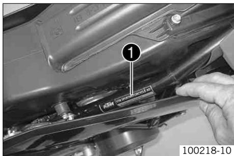
Type label ❶ is located on the upper right frame tube below the seat.
