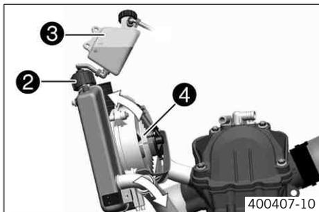
The coolant is cooled by the air stream and a radiator fan ④, which is controlled by a thermostat.
