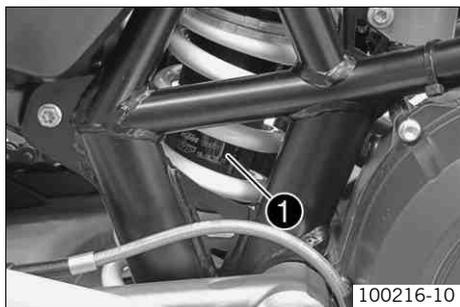
The shock absorber part number ❶ is on the right of the shock absorber.
