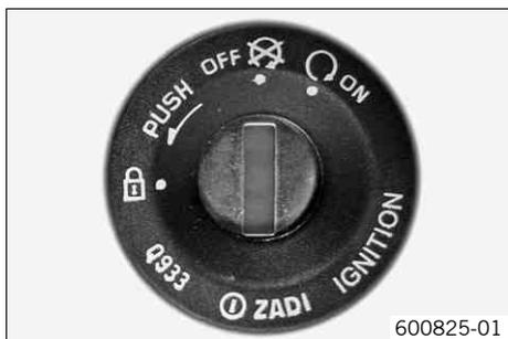
The ignition/steering lock ❶ is in front of the upper triple clamp.
