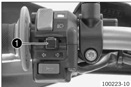
The flasher switch ❶ is fitted on the left side of the handlebar.
