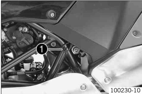
The seat can be released using strap **1**.
