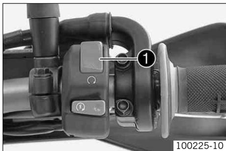
The emergency OFF switch ❶ is fitted on the left side of the handlebar.
