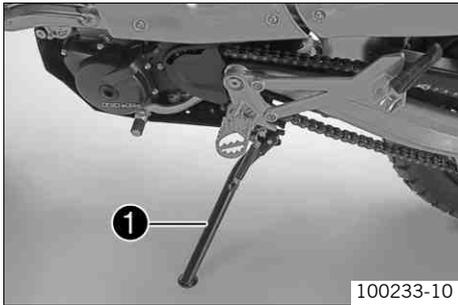
The side stand ❶ is coupled with the safety electric starter system - see the riding instructions.
