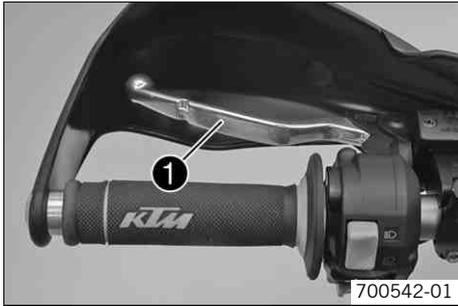
The clutch lever ❶ is fitted on the left side of the handlebar.
