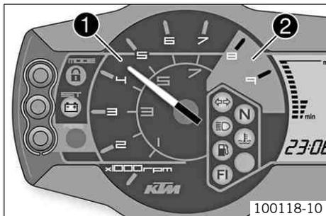
The tachometer ❶ shows the engine speed in revolutions per minute.
