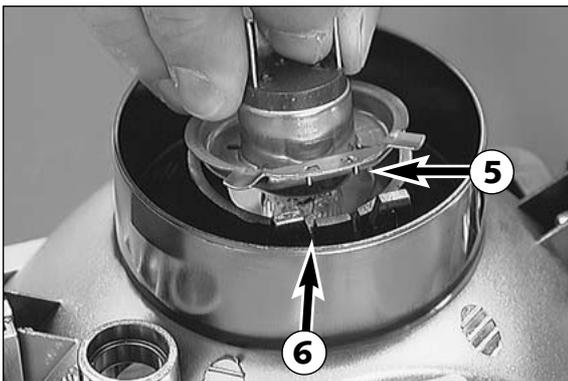
Insert the new lamp such that the noses **5** engage in the recesses **6**. When doing so, do not touch the glass body of the lamp so that it remains free from fat. Engage retaining clip, mount rubber cap and connector. If the parking-light lamp is to be replaced, simply insert it in the holder. Reinsert the parking-light lamp together with the holder. Engage the bottom end of the headlamp mask at the retaining pins and fix the mask by means of the rubber bands.
