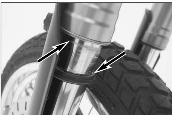
Clean dust-protection bellows, outer tubes, and fork tubes thoroughly, and oil them thoroughly with silicone spray. Then, push dust-protection bellows into the outer tubes by hand.
