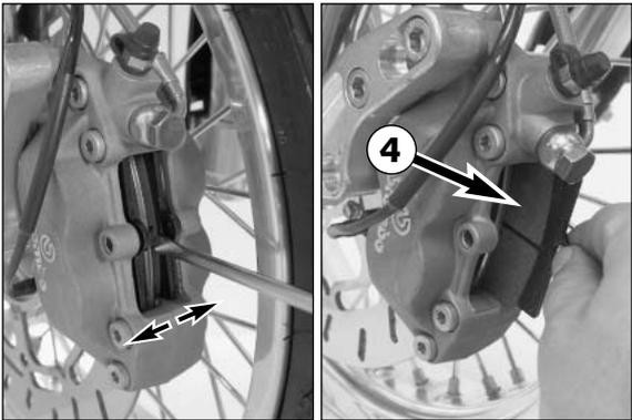
Mount both brake pads and position the locating spring. Push the bolt all the way in and mount the retainer.
