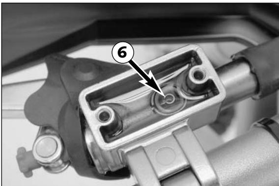
Having completed the bleeding procedure, you have to verify that the oil level in the master cylinder is correct. If necessary, fill up with biodegradable hydraulic oil SAE 10 (e.g. Shell Naturelle HF-E15). Biodegradable hydraulic oil is available from your KTM dealer (50ml).
