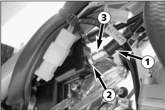
To adjust the throttle cables, dismantle the seat and the tank together with spoilers. Slide back the protection cover ①. Loosen the counter nut ② and turn the adjusting screw ③ accordingly. Turning the adjusting screw counterclockwise will reduce the backlash, turning the adjusting screw clockwise will increase the backlash.
