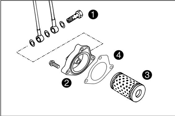
Place the new oil filter ③ on the connection in the oil filter cover and mount together with a new seal ④. Tighten the 3 screws in the filter cover to 5 Nm. Tighten the hollow screw with seals and tighten to 15 Nm. Finally, start the engine and check the oil system for leakage.
