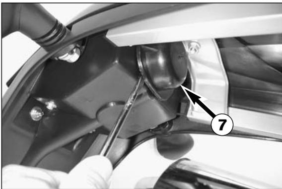
**Exchanging the brake light and tail light bulb**
