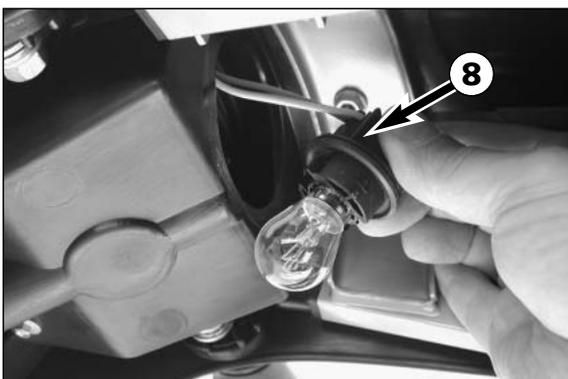
Turn the lamp socket **8** approximately 30° counterclockwise and pull it out of the tail light housing. Slightly depress the bulb, turn it approx. 30° counterclockwise and pull it out of the socket. To mount the lamp reverse the worksteps indicated above.
