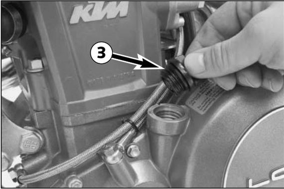
Clean the plugs thoroughly with a fireproof solvent and compressed air, in order to remove the metal abrasion. After all the oil has drained through, clean raised and flat faces and install plugs with seals. Tighten plug 1 with 30 Nm and plugs 2 with 20 Nm.
