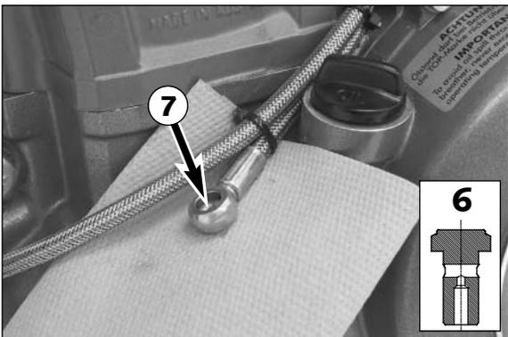
It is necessary to bleed the micro filter so that all friction areas can be quickly supplied with engine oil. To do this, fill with oil and remove the jet screw 6 from the oil line on the clutch cover. Start the engine and close off the oil filler hole on the clutch cover with a rag. Allow the engine to run at idle until oil runs out of the oil line 7. Turn the engine off. Install seal rings and the jet screw. Torque the jet screw to 10 Nm and check for leaks.
