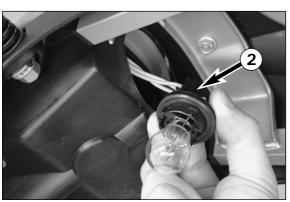
Turn the lamp socket 2 approximately  $30^\circ$  counterclockwise and pull it out of the tail light housing.
