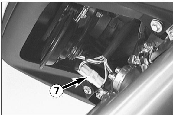
When the battery of the motorcycle is empty the engine can only start by disconnecting the power supply of the head light. For this purpose a pin and socket connector
