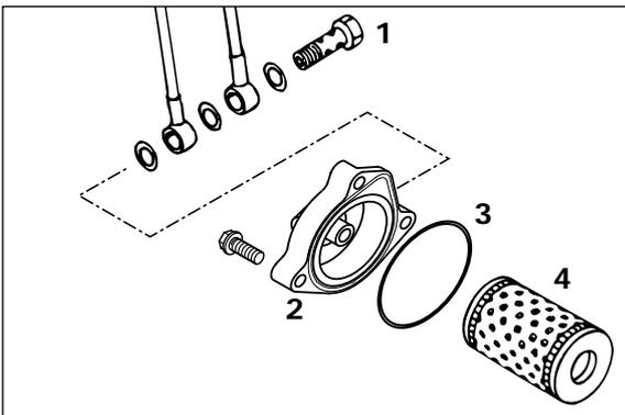
Check the O-ring **3** for damage. O-rings need not be replaced unless damaged. Press the O-ring into the groove of the filter cover. Fit new oil filter **4** with rubber gasket on the fitting in oil filter cover and mount cover with filter. Mount three screws and tighten with 5 Nm (4 ft.lb). Mount hollow screw with seal rings and tighten with 15 Nm (11 ft.lb). Start engine and check oil system for leakage.
