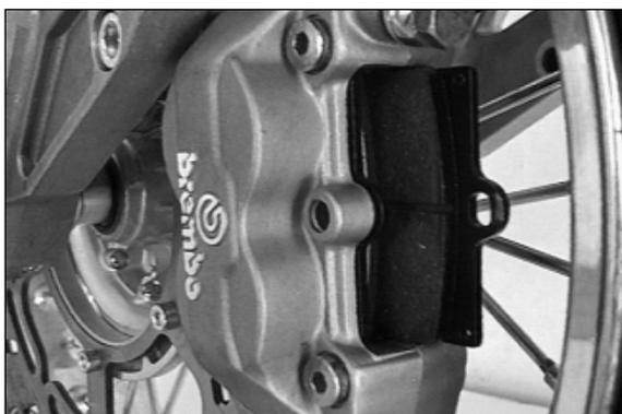
Insert new brake pads into the brake caliper, replace retainer spring (arrow pointing upward), and reinsert cotter pin. Hammer the bolt into the caliper as far as it will go and replace cotter pin.
