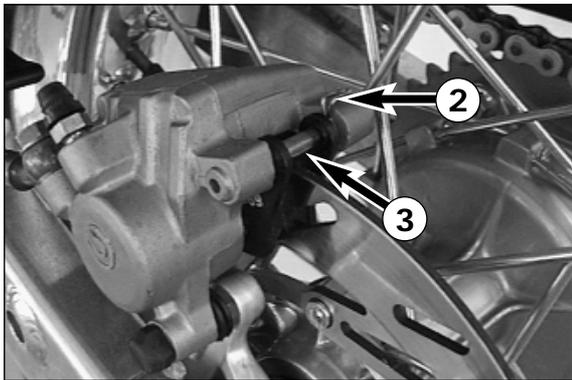
Remove cotter pin ②, knock out the cotter bolt ③ from the brake caliper with an insert stake towards the chain wheel and remove brake pads. Carefully clean the brake caliper with compressed air and check sleeves of the guide pins for damage.
