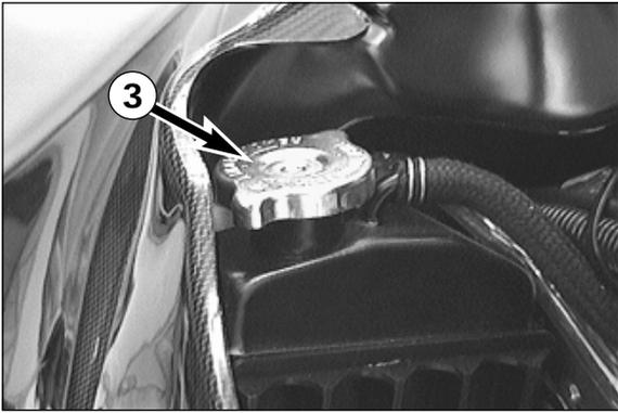
A mixture of 40% antifreeze and 60% water is used as cooling liquid. However, the anti-freeze protection must be at least -25° C (-13° F). Aside from antifreezing protection, this mixture also provides great corrosion protection which is why it must not be replaced by pure water.
