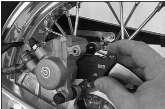
Slide right brake pad into the brake caliper and fix it with the bolt. Slide in the left brake pad and knock in the bolt to end position. Mount safety device ②.
