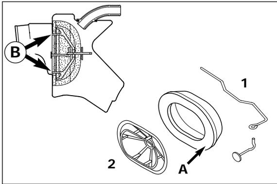
Mount the air filter on the filter support 2. Grease the front side A of the filter, to improve the seal. Mount the air filter and the filter support in the filter box. Make sure they are centered B, and lock into place with the filter bracket 1.
