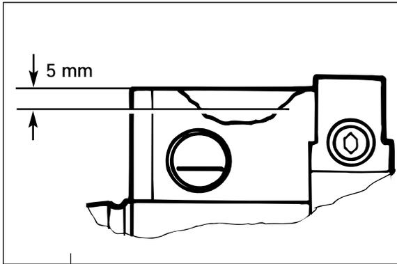
Place hand brake cylinder in a horizontal position and fill the brake fluid reservoir to 5 mm below the rim with brake fluid (DOT 5.1). Replace membrane and lid, tighten screws. Rinse off spilled or overflowing brake fluid with water.
