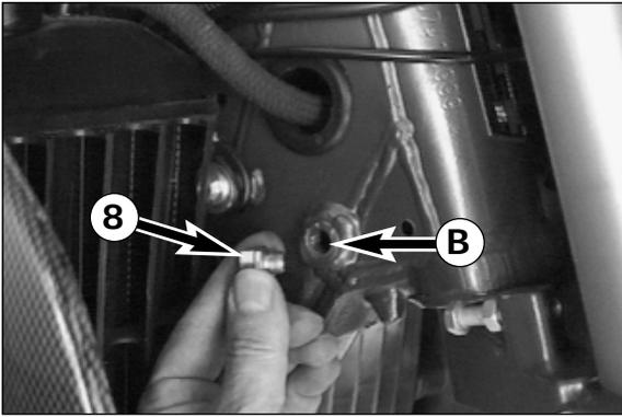
To allow the air to escape from the front pipe of the frame, remove plug **8** next to the steering head. Start engine and let it run in idle (1-2 minutes) until oil escapes at the bore **B**. As soon as oil starts to escape, turn off the engine, and mount plug together with the gasket.
