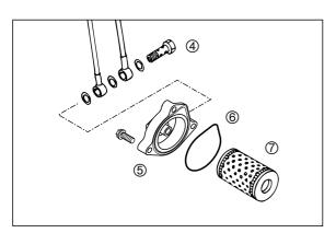
Check the O-ring 6 for damage. O-rings need not be replaced unless damaged. Press the O-ring into the groove of the filter cover. Fit new oil filter with rubber gasket on the fitting in oil filter cover and mount cover with filter. Mount three screws and tighten with 5 Nm (4 ft.lb). Mount hollow screw with seal rings and tighten with 15 Nm (11 ft.lb). Start engine and check oil system for leakage.
