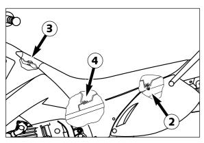
To mount the seat hook it into the oval head screw, lower the rear part of the seat and push the whole seat forwards. If necessary push the middle of the seat slightly down to let the retaining bracket ② engage with the seat. Finally fasten the seat with the corresponding screw.
