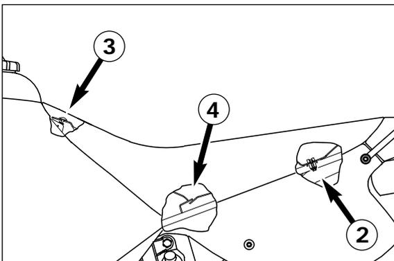
To install the seat, hook the seat into the oval-head screw, set the rear portion down on the frame, and slide it forward. If necessary, press down on the front area of the seat so that the seat catches on the retaining bracket ④. Insert and tighten the collar screw.
