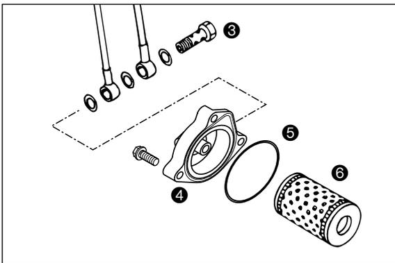
Check the O-ring ⑤ for damage. O-rings need not be replaced unless damaged. Press the O-ring into the groove of the filter cover ④. Fit new oil filter ⑥ with rubber gasket on the fitting in oil filter cover and mount cover with filter. Mount three screws and tighten with 5 Nm (4 ft.lb). Mount hollow screw ③ with seal rings and tighten with 15 Nm (11 ft.lb). Start engine and check oil system for leakage.
