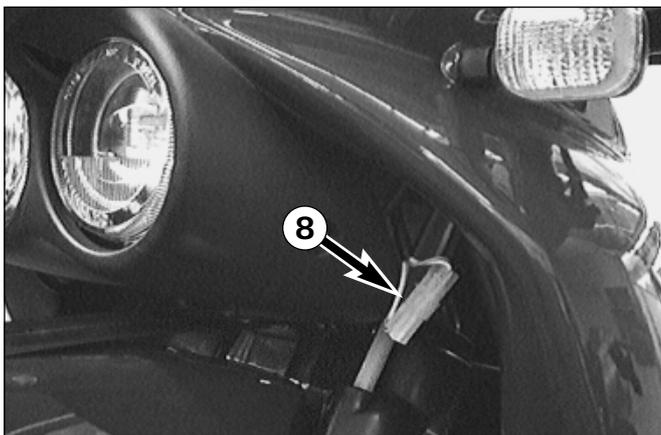
When the battery of the motorcycle is empty the engine can only be started by disconnecting the power supply of the head light. For this purpose a pin and socket connector ❸ can be found below the headlight mask on the lefthand side. Disconnect the pin and socket connector and start the engine with the kickstarter
