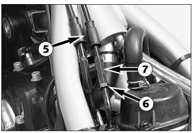
If a correction is necessary, start by removing the tank. Slide back the protection cover **⑤**. To set the backlash, loosen the counter nut **⑥** and turn the adjusting screw **⑦** accordingly. Then, fasten the counter nut and slide the protection cover back on.
