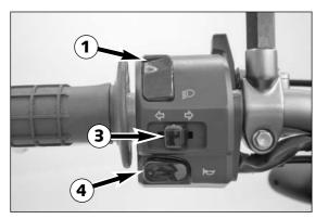
←⇒ The indicator switch ③ returns to central position after actuation. Press flasher switch towards switch housing to switch off the flasher.
