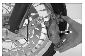
After mounting the front wheel, slide the brake caliper to the brake disc. Remove the grease from the threads of both screws 4 and apply Loctite 243. Tighten the screws with 40 Nm.
