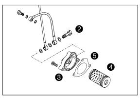
Place the new oil filter **3** on the connection in the oil filter cover and mount together with a new seal **3**. Tighten the 3 screws in the filter cover to 5 Nm. Tighten the hollow screw with seals and tighten to 15 Nm. Finally, start the engine and check the oil system for leakage.
