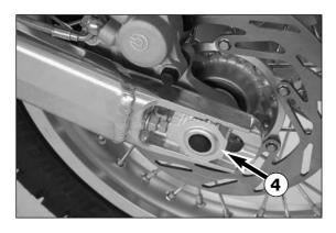
NOTE: The large adjusting range of the chain adjusters 32mm (1.28 in) allows you to use different secondary ratios in combination with the same chain length. The chain adjusters **4** can be rotated by 180°.
