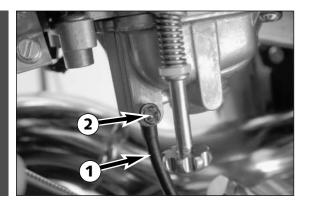
Open the drain plug ② (turning it counterclockwise) by several turns, and drain the fuel from the float chamber.
