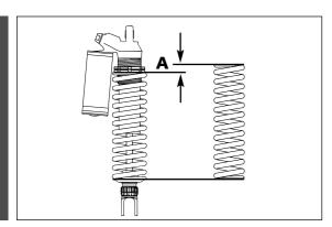
Loosen the locking ring • with the hook wrench from the tool set. Change the spring preload with the adjusting ring • and retighten the locking ring.
