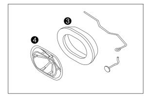
Mount the air filter on the filter holder, position in the filter box (make sure to center) and fix with the retaining clip. Check whether the air filter is positioned correctly and mount the filter box cover.
