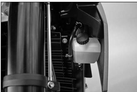
If necessary, pour cooling liquid into the radiator up to the upper edge of the filler neck, mount the radiator cap and rest the motorcycle on the side stand again. Fill the compensating tank with cooling liquid until it reaches a level between the MIN and MAX mark. Close the compensating tank.
