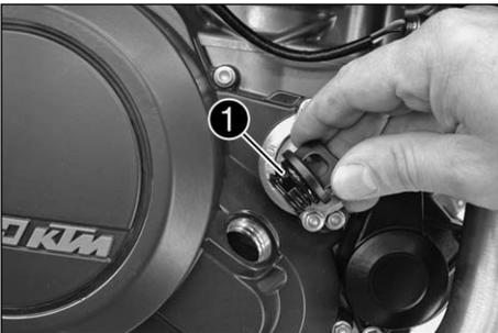
Unscrew the plug [1]. Add 2 liters (0,53 USgal) of fully-synthetic 10W/60 engine oil according to JASO MA quality requirement (e.g. Motorex Cross Power 4T 10W/60) and remount the plug. Start the engine and allow to run warm in neutral until 5 bars on the temperature indicator light up. Switch off the engine and check the engine oil level (see "Checking the engine oil level").
