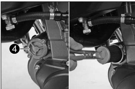
Remove the oil filter cover [4] and pull the oil filter out of the engine case with circlip pliers (upside-down).
