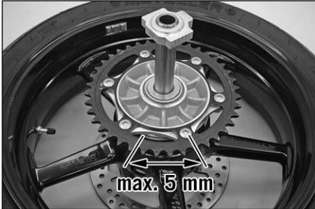
For this purpose, lie the rear wheel on a work bench with the rear sprocket upwards, and put the wheel spindle in the hub. Now hold the rear wheel firmly and try to turn the rear sprocket. The rear sprocket may not turn more than maximum 5 mm (0,2 in) measured on the outside. If the play in the chain wheel is larger, all 6 shock absorption rubbers are to be replaced.
