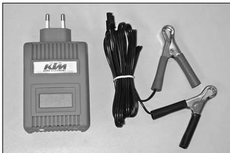
To charge the battery while mounted, always use the KTM battery charger (Item no. 58429074000) to ensure that the electric system is not damaged by excess voltage. **Always remove the battery if using other battery chargers!** You can also use this charging device to test the off-load voltage and startability of the battery and generator. It is impossible to over-charge the battery with this device.
