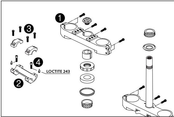
For this purpose, remove screws ③ of the handlebar clamps and screws ④ of the handlebar support. Position handlebar support, apply Loctite 243 and tighten screws ④ to 40 Nm (30 ft.lb). Mount handlebar and handlebar clamps, and tighten screws ③ to 20 Nm (15 ft.lb). The gap between handlebar support and handlebar clamps is to be of equal size in the front and in the rear.
