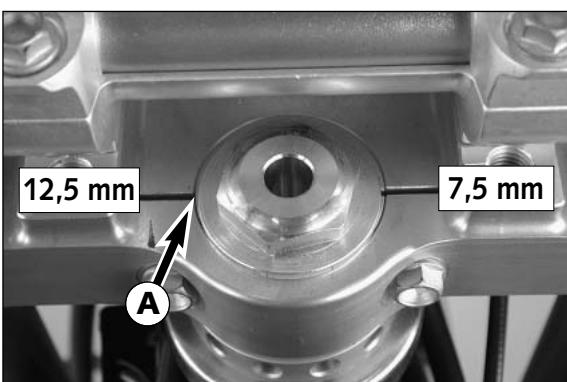
If the groove A is on the left, the offset is 12.5 mm and the caster 97.4 mm. This setting will give you better handling in curves.
