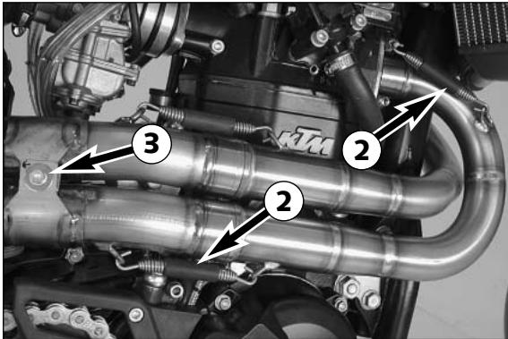
Remove the manifold by detaching both springs ② and screw ③.
