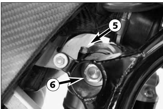
To change the height of the tail end, loosen the clamping screws ⑥. Place a 19 mm socket wrench on the HH screw ⑤ and turn the eccentric accordingly. Do not turn the eccentric more than 90 ° up or 90 ° down from the standard position. The adjustment range is ± 24 mm on the rear wheel. Tighten the clamping screws to 25 Nm.
