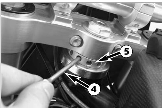
The steering head bearings should be regreased at least once a year (i.g. Motorex Long Therm 2000)
