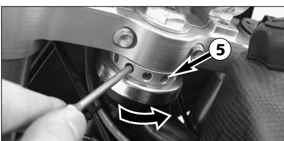
To adjust, loosen the clamping screws 5 on the fork stabilizers. Insert a pin (6 mm) in the adjusting nut 6 and turn the fork tube 180° in a counter-clockwise direction (not clockwise or you will change the positioning of the steering head bearings). The groove A must match the slot on the upper triple clamp. Tighten the clamping screws to 20 Nm.
