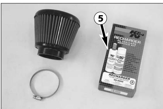
Rinse the air filter thoroughly with a special cleaning fluid and allow to dry. Oil the dry air filter with K&N filter oil. Also clean the air filter box. Check the carburetor connection boot for damage and a tight fit.
