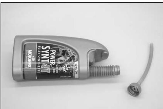
To facilitate bleeding of the oil system, we have added a hose connection piece and a plastic hose to the set of tools. Take an empty oil can (1 liter) and drill a 7 mm (0.28 in) -diameter hole into the lid. Screw the hose connection piece into the lid from the outside, and secure it from the inside with the M8 hexagon nut.
