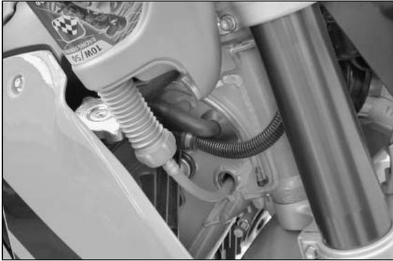
Let the motor run until it warms. Check the oil drain plugs and the fine screen filter to make sure they are properly sealed. Check the level of the motor oil. Place the motorcycle on a horizontal surface (main stand) and wait for 5 minutes. Checking the oil level, he should be between the two marks on the inspection glass, however, it must never rise above the MAX mark. Otherwise, engine oil would get into the air filter box by way of the engine venting system. Add engine oil, if necessary.
