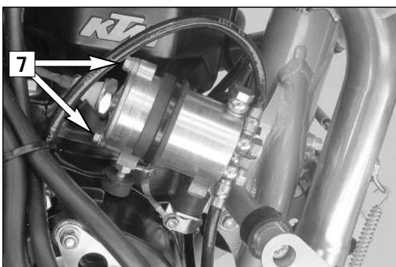
Remove the right front fuel tank. Loosen the two HH screws [7] and remove the microfilter cover.
