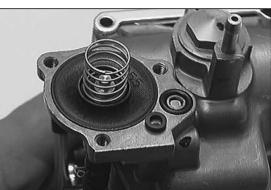
Turn the carburetor around, remove the 3 screws and remove the cover of the accelerator pump.
