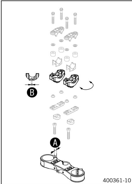
On the upper triple clamp, there are 2 holes at a distance of **A** to each other.
