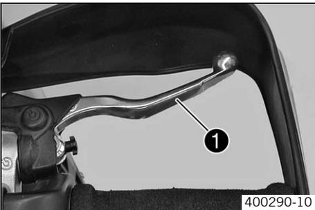
The hand brake lever ❶ is located on the right side of the handlebar and operates the front wheel brake.
