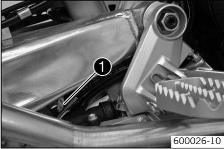
Shock absorber part number ❶ is attached at the shock absorber unit, to the rear of the direction of travel.
