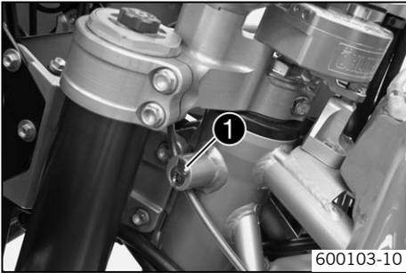
The steering lock ❶ is fitted on the left of the steering head. The steering lock is used to lock the steering. Steering, and therefore riding, is no longer possible.
