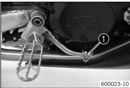
The foot brake pedal ❶ is located in front of the right footrest and operates the rear wheel brake.
