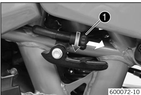
The chock knob ❶ is fitted on the left side of the frame.
