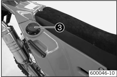
The rear fuel tank is filled via filler cap ③. This model has three separate fuel tanks controlled by a fuel tap. Two fuel tanks are located in front of the seat and one fuel tank is located beneath the seat.
