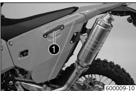
There is one handrail ❶ attached at the left and one at the right (at the rear tank). The handrail is used for shunting the motorcycle.
