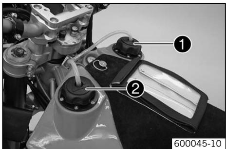
The right fuel tank is filled via filler cap ① and the left fuel tank is filled via filler cap ②.
