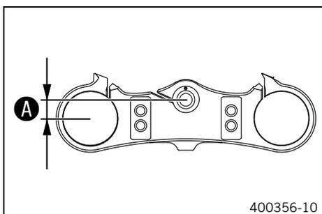
The fork offset A has an impact on the handling of the vehicle. It is calculated from the center of the fork leg to the center of the steering head bearing. The fork offset can optionally be adjusted.
