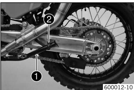
To park the motorcycle, remove the rubber band ❷, fold down the side stand ❶ with your foot and rest the motorcycle against it.
