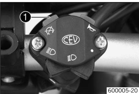
The short circuit button ❶ is fitted on the left side of the handlebar and has no function upon delivery.
