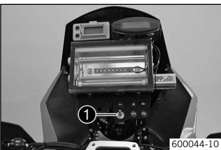
The ignition switch ❶ is located to the left of the indicator lamp on the instrument support.
