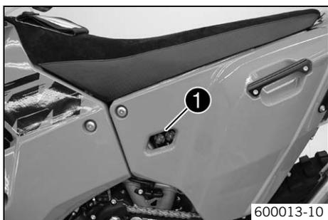
The compression damping can be adjusted via an opening ❶ on the left side of the rear tank.
