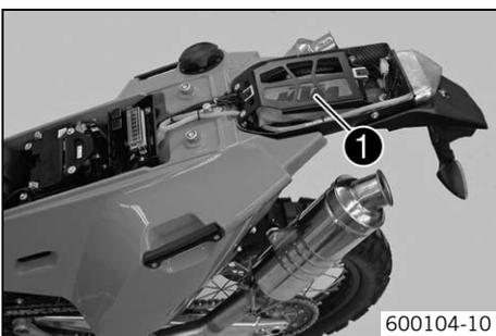
The tool set ❶ is contained in the accessories box and can be stored in the compartment beneath the additional lamps.
