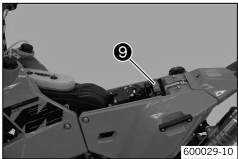
The fuse box ⑨ is located under the seat.
