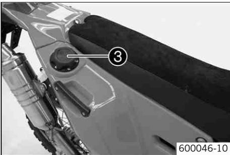
The rear fuel tank is filled via filler cap ❸.
