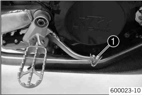
Foot brake pedal ❶ is located in front of the right footrest. The rear brake is engaged with the foot brake pedal.
