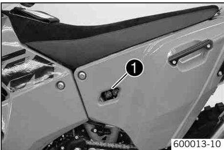
The compression damping can be adjusted via opening ❶ on the left side of the rear tank.
