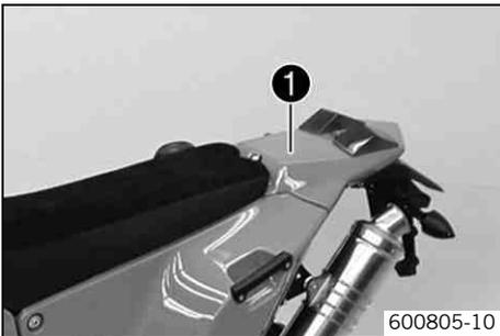
The tool set is contained in the accessories box and can be stored in compartment ❶ beneath the additional lamps.
