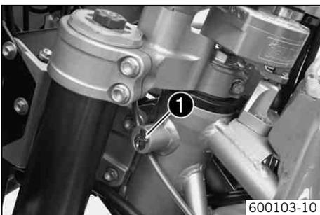
The steering lock ❶ is fitted on the left of the steering head.
