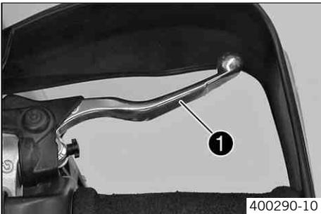
The hand brake lever ❶ is fitted on the right side of the handlebar. The front brake is engaged using the hand brake lever.
