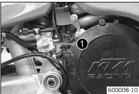
Fuel tap ❶ is located on the right over the fork pivot. The fuel tap can be used to control the individual fuel tanks. The fuel tap does not have an **OFF** position since the fuel pump does not let fuel pass when the engine is stopped.
