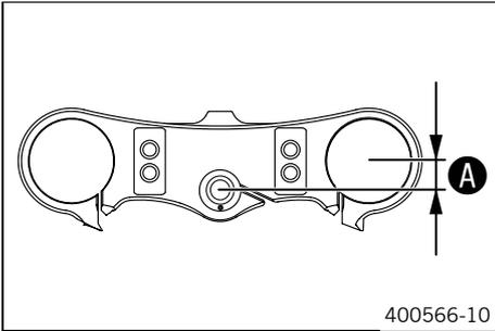
The fork offset **A** has an impact on the handling of the vehicle. It is calculated from the center of the fork leg to the center of the steering head bearing.
