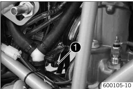
The idle speed is adjusted with the adjustment screw ②.
