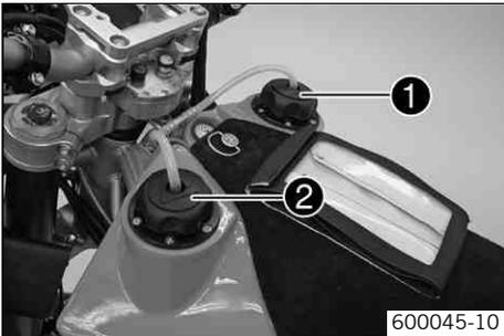
The right fuel tank is filled via filler cap ❶ and the left fuel tank is filled via filler cap ❷.
