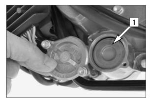
Insert a new oil filter [1] in the engine case, grease the O-ring and mount the oil filter cover together with the O-ring. Tighten the screws to 6 Nm.
