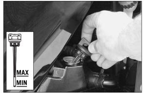
The oil level should fall between the lower end of the oil dipstick (MIN) and the MAX mark.
