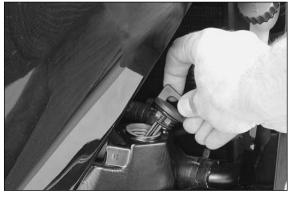
Add 2.5 liters (0.7 USgal) of fully synthetic engine oil meeting the JASO MA standard (e.g. Motorex Power Synt 4T) and mount the oil dipstick. Start the engine, allow to run warm for 4 minutes and switch off the engine. Remove the oil dipstick and add engine oil up to the MAX mark (approx. 0.5 liters, 0.13 USgal).
