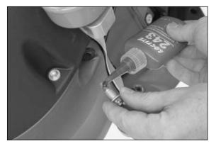
Apply Loctite 243 to the thread of the 4 screws, mount the underride protection and tighten the screws to 25  $\mbox{Nm}.$
