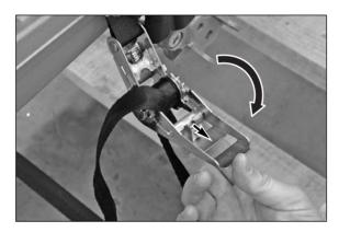
NOTE: to loosen the tensioning strap, first pull the lock towards the outside (away from the drum; small arrow) and then fold the handle down.
