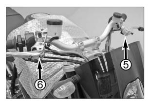
NOTE: align the control elements and handlebar; run the hoses and wiring harnesses as illustrated.
