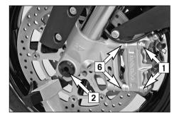
Remove the screws [1] on the left and right brake caliper and carefully pull the brake calipers and bushings [6] off the brake disks towards the back.
