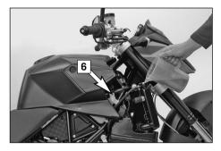
To completely bleed the cooling system, the motorcycle must be raised approx.  $50\ \text{cm}$  ( $20\ \text{in}$ ) in the front.
