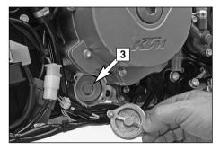
Insert a new oil filter [3] in the engine case, grease the O-ring and mount the oil filter cover together with the O-ring. Tighten the screws to 6 Nm.
