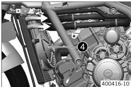
Cooling takes place by means of the air stream and a radiator fan ❹, which is controlled by a thermoswitch.
