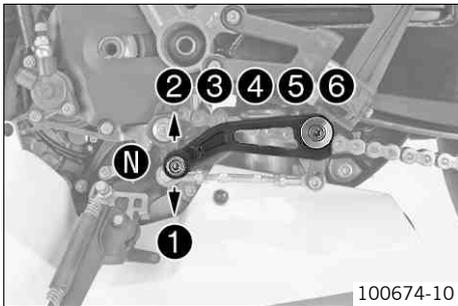
The gear positions can be seen in the picture.
