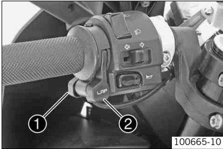
The **MODE** button ❶ is fitted on the handlebar, front left.
