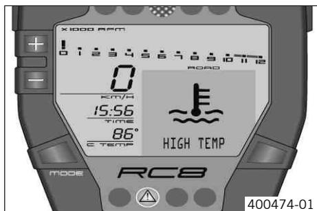
**HIGH TEMP** appears on the info display if the coolant temperature rises above the specified value.
