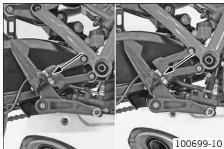
The adjustable footrest system enables an individual setting of the footrest height and an individual adjustment of the operating elements. The lower footrest position enables a more comfortable knee angle, the upper footrest position a sporting sitting position and more forward-leaning freedom for use in racing.
