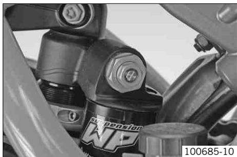
The shock absorber can regulate compression damping separately in the low and high speed ranges (Dual Compression Control). The term low and high speed refers to the movement of the shock absorber during compression and not the riding speed of the motorcycle. Changes in the low-speed range settings have an impact on the high-speed range and vice versa.
