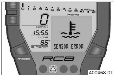
**SENSOR ERROR** appears on the info display if the discrepancy between the front and rear cylinder coolant temperature sensor values differs by more than the specified value.
