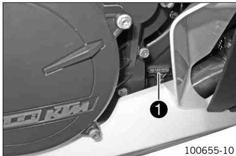
The engine number ❶ is stamped on the right side of the engine.
