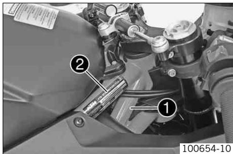
The vehicle identification number ❶ is stamped on the frame behind the steering head on the right.
