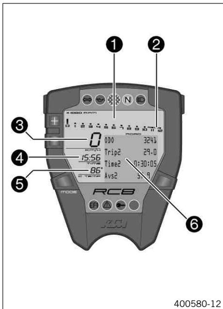
The tachometer **1** displays the engine speed in revolutions per minute (RPM).
