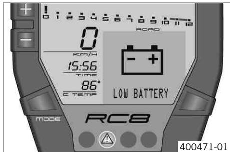
**LOW BATTERY** appears on the info display if the battery voltage falls below the specified value.
