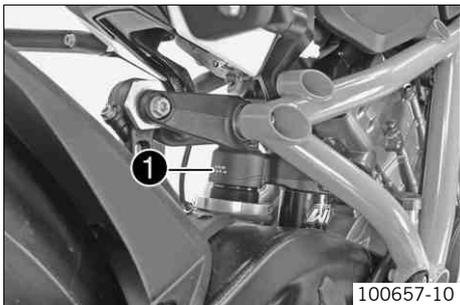
The shock absorber part number ❶ is stamped on the upper part of the shock absorber above the adjusting ring towards the rear.
