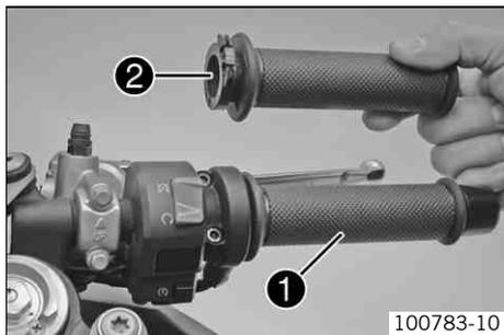
The installed throttle grip ❶ twists opens uniformly (linear) over the entire range of the throttle valve.
