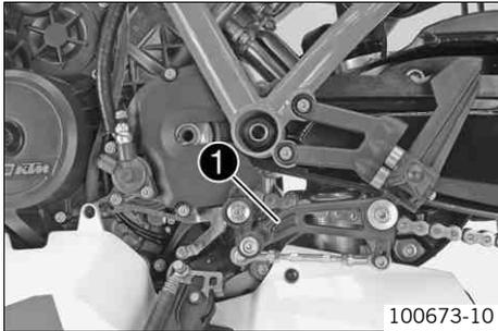
The shift lever ❶ is mounted on the left of the engine.
