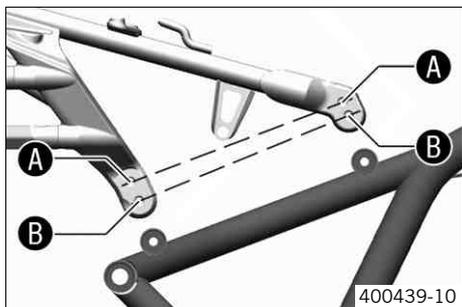
The frame rear height can be set to two different positions, enabling ergonomic adjustment of the seat height.
