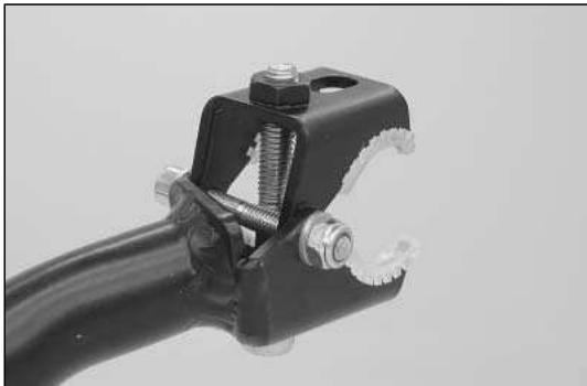
Partially screw in all of the screws. Do not tighten until all screws are partially screwed in.
