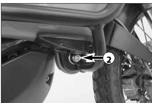
Screw the bar on the side of the tank using the M8x70 AH screws and one washer ② each.
