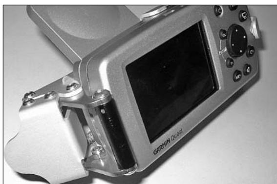
To place the unit in the bracket, pull the lever all the way out. Slide the unit with the antenna extended under the right hook and gently press into the bracket. Let go of the lever and press down until the lock is at a right angle to the bracket. If the bracket is lockable, you can lock the bracket now. Warning for lockable brackets: the bracket is not 100% theft-proof. Never leave your unit unattended. Remove the unit from the bracket whenever you leave your vehicle.
