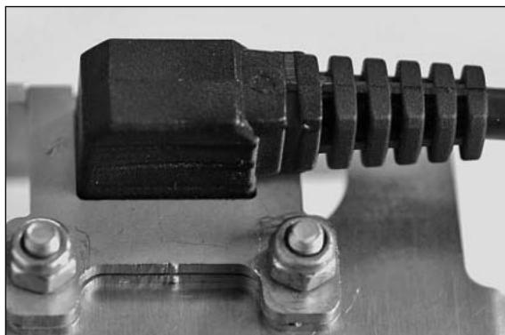
Now insert the connector in the recess from below and fasten with the M3 x 10 flat-head screws and self-locking nuts. The cable will lead out of the bracket to the right. Screw the base plate back on and mount the bracket to the vehicle. Connect to positive lead after the ignition lock. Mount the bracket to the center rail on the handlebar or to a suitable adapter using the pipe clamp attached to the bottom of the bracket.
