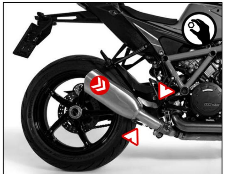
Align the REMUS sport exhaust and tighten the connections.
