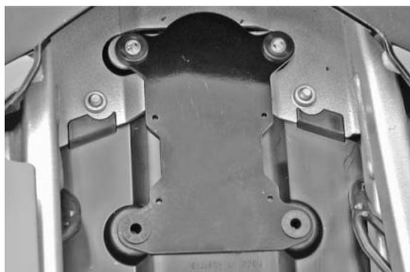
Screw on the mounting bracket, using the M5x16 collar screws and A5.3 washers in the rear and the M5x20 collar screws in the front.
