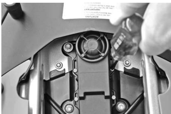
Connect the alarm system to the wiring harness. Slide the grommet on the wiring harness over the connector. Screw the alarm system onto the mounting bracket using the four 3.5x16 oval head self-tapping screws.
