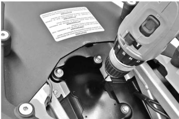
Carefully drill through the four holes on the mounting bracket through the storage compartment using a 2.5 mm bit. Do not drill down too deeply to keep from damaging the fender.
