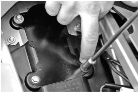
If the rubber grommets turn while turning in the screws, hold them in place with your finger, as shown in the photo. Carefully tighten the screws until the mounting bracket is firmly seated.
