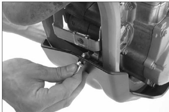
Mount the engine guard with the hanger between the engine and the frame and bend it upwards towards the front. Fix the engine guard with the quick-release fastener on the fixing bracket with a quarter-turn and tighten the HH screws of the fixing bracket.
