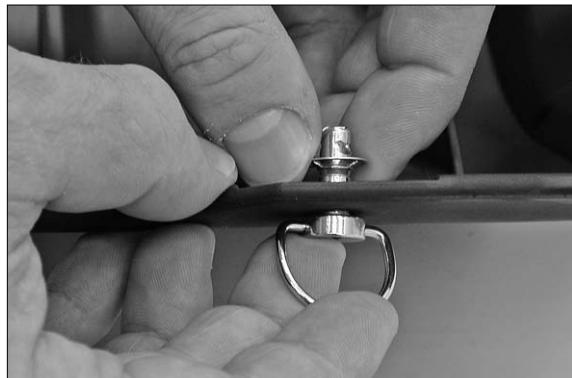
Push the quick-release fastener from the outside through the bore on the engine guard and push the lock ring from inside over the quick-release fastener until it locks in place.
