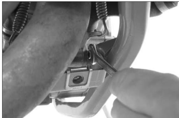
Mount the fixing bracket with the HH screws and nuts on the frame. Do not over-tighten the screws, but check that the bracket can still move.
