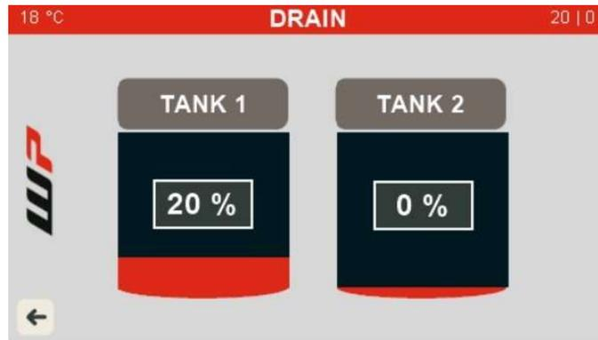
3. Connect the hose via a quick connector to the desired internal tank connector that you want to drain – “TANK 1” or “TANK 2”.
