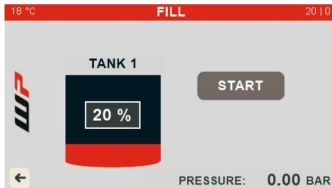
7. Select “START” and press OK. Filling process will start once the vacuum reaches -0.7 Bar.
